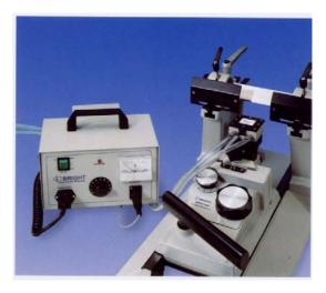
Pictured above the Solid State Freezer is connected to the Bright 8000 Retracting Base Sledge Microtome and below is connected to the Bright 5040 Rotary Retracting Microtome.
