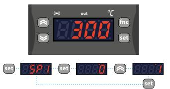
Once the 'SP1' label has been displayed, press the "set" button to display the Set point 1 value. The Set point value appears on the display. To change the Set point value, use the "UP" and "DOWN" buttons within 15 seconds.
