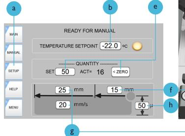
f. Using a ruler, estimate the stroke length between the knife's edge and just before the specimen. This measurement should leave the knife short of the specimen so the machine can then change from rapid speed to the set cutting speed. If knife is not fitted you can use the knife holders pivot point that is marked with a pink dotted line in the image.
