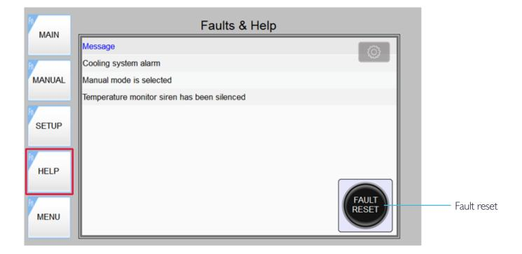
Note: Is for the Top level user/ service engineer to access the diagnostics and master settings.
