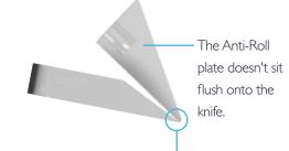
Start with roll plate point below the point of the knife and advance it forward while sectioning until sections slide underneath plate. c. Place the Anti-roll plate back against the knife and start to cut sections. If the plates edge is too far back in relation to the knife edge the sections will curl up on the tip of the knife.
