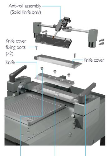
Knife fixing bolts (x3) Knife holder Clamping Handle
