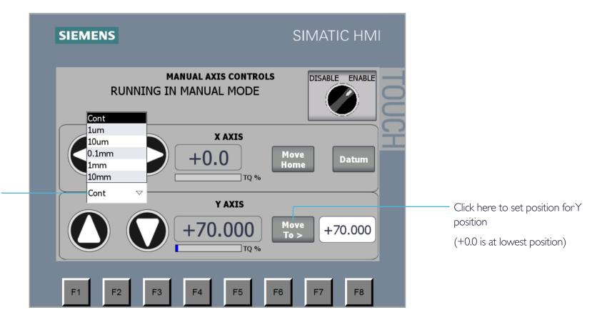
These values allow the user to select the travel distance for each press of any of the directional buttons, "Cont" stands for Continuous mode where movement occurs for as long as the button is pressed
