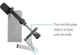
Start with roll plate point below the point of the knife and advance it forward while sectioning until sections slide underneath plate.
