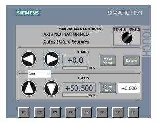
i. On the touchscreen press and hold the Datum button until Datum complete message shows (If Motor's inhibited light is illuminated press the white Start button to activate them to allow Datum function).
