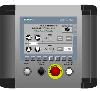
The X axis value should read +0.0 when at datum point.
