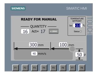
n. Once the parameters are set, return to the main screen (F1) and run the cycle, this can be done in either single cut or continuous cut mode.
