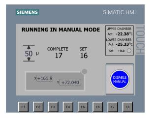
m. Go onto the set-up screen (F4) to set parameters for the initial trimming cycle. (Click on the values to edit).
